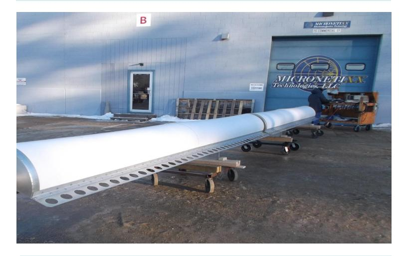
The antenna is built in two sections, and bolts together in the middle. The radome system wraps around the front two-thirds of the antenna, covering the vertical polarizer elements. Bay count? 6 And with each bay being 65 inches long, the length of the antenna comes out to about 33 feet. The antenna uses a 3-1/8" EIA input, so the input power rating is 25 kW.
